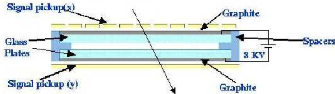
A passing charged particle induces an avalanche, which develops into a spark. The discharge is quenched when all of the locally available charge is consumed.
