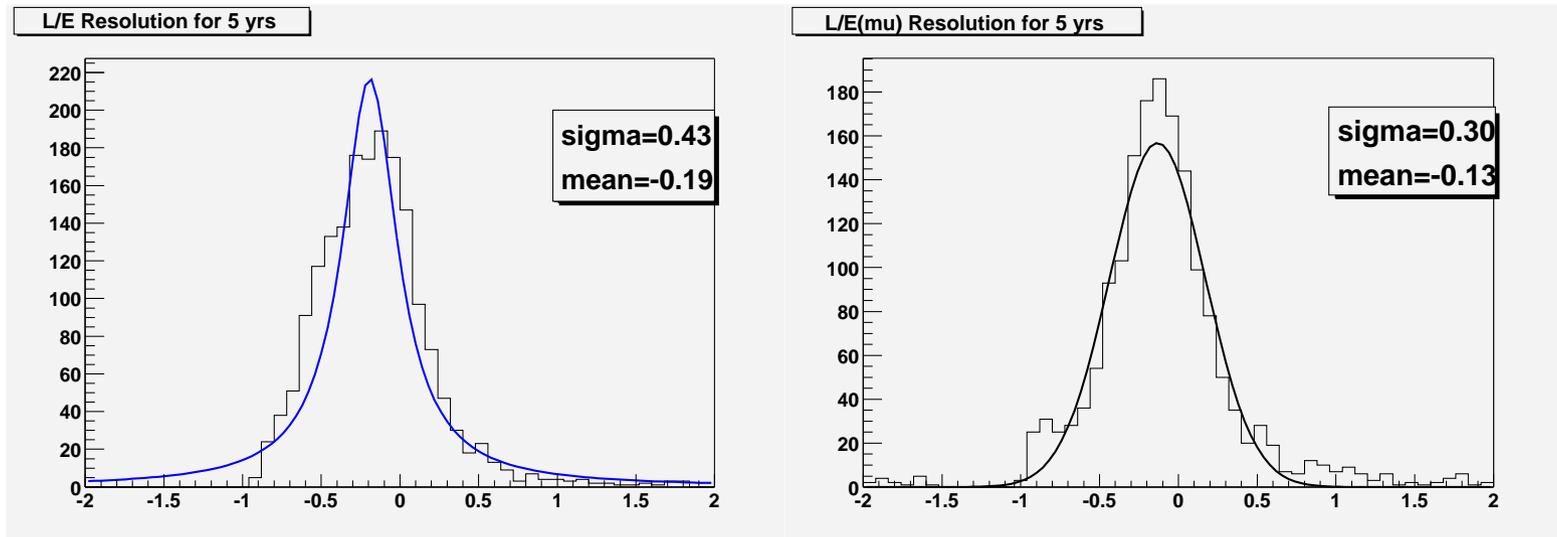
$L/E$  resolution from reconstruction (left); muon only (right).
