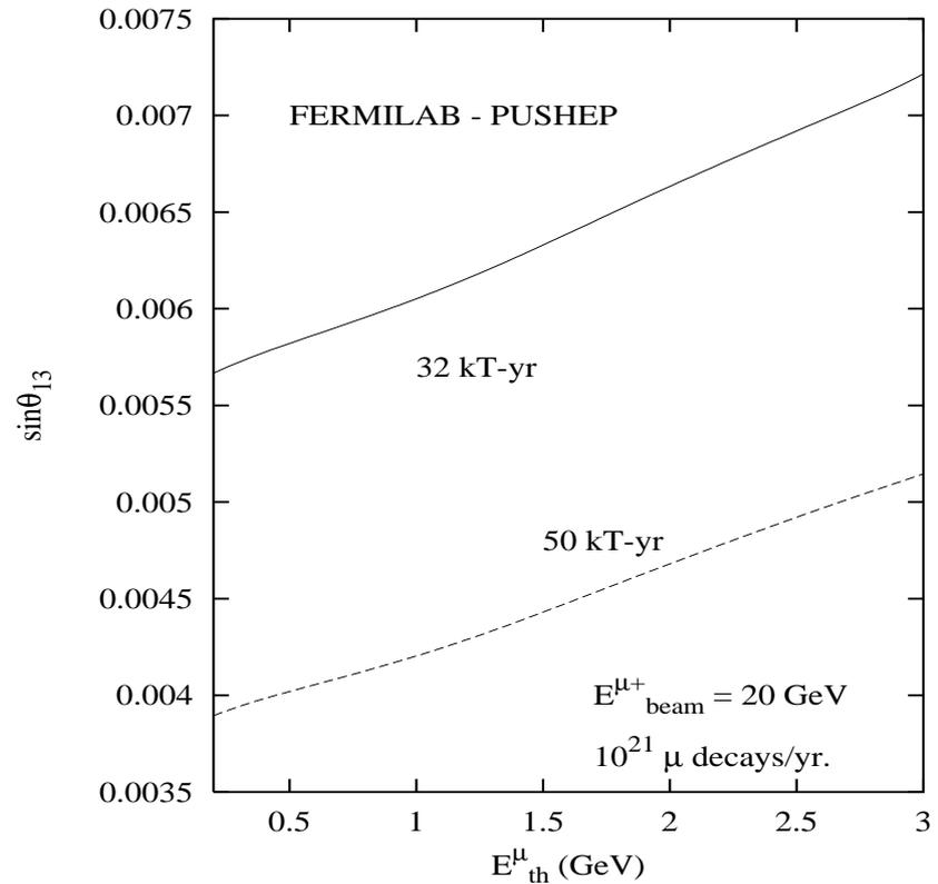
$\sin \theta_{13}$  reach for different muon threshold energies.
