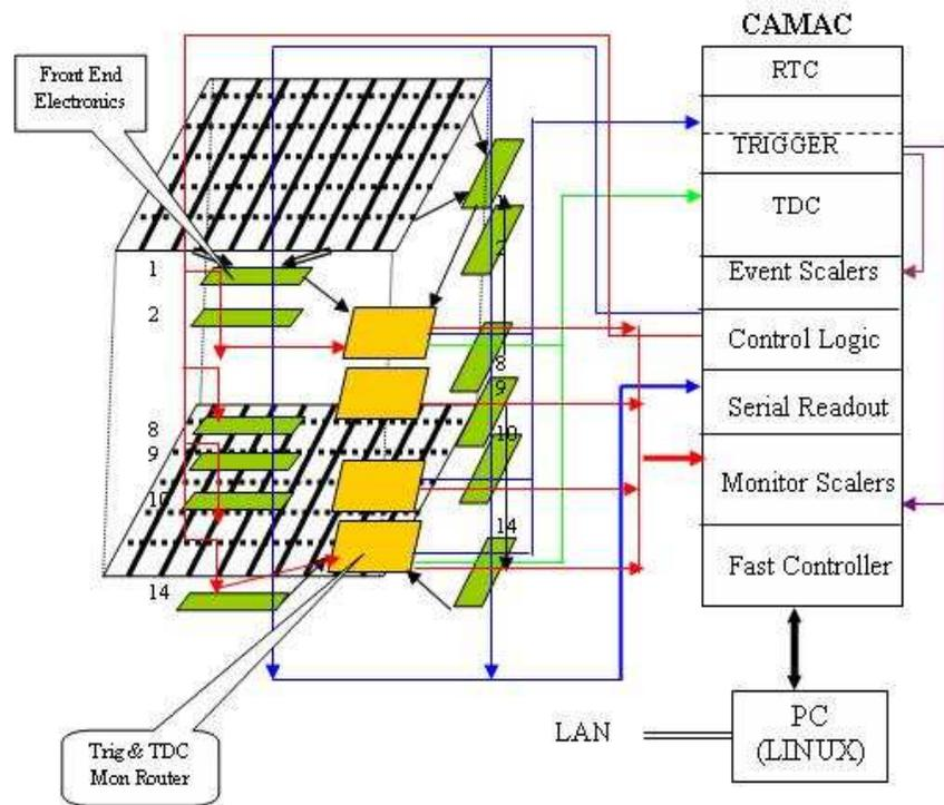
A schematic of the read-out electronics for the prototype
