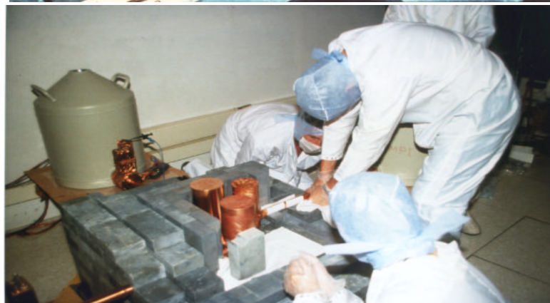
Fig. 2 The \beta\beta -laboratory of the HEIDELBERG-MOSCOW experiment in the Gran Sasso and its location between halls A and B, and four of the enriched detectors during installation (from top to bottom).
