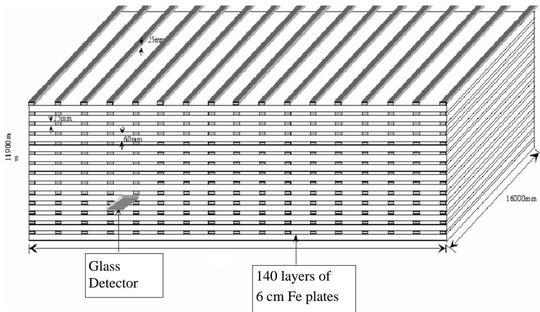
Figure C-4: Schematic view of ICAL including structural supports.
