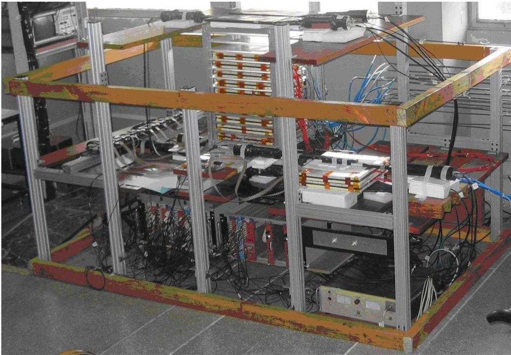
Figure 5.16: Muon tracking setup using RPC stack.
