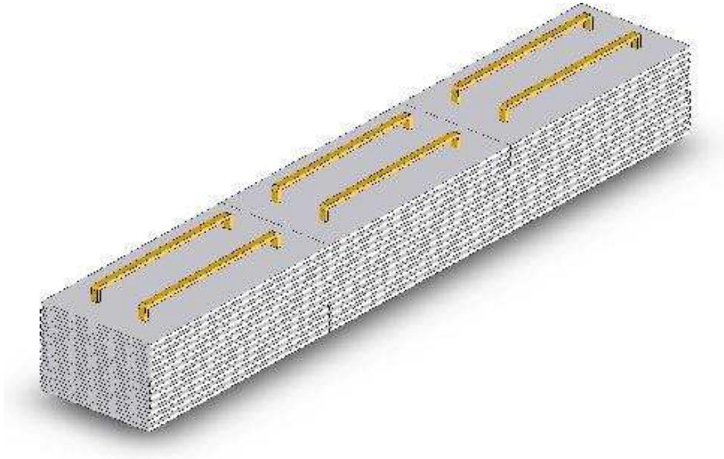
Figure 5.32: Layout of the coils (longitudinal) in Helmholtz-like pair design of the ICAL magnet.
