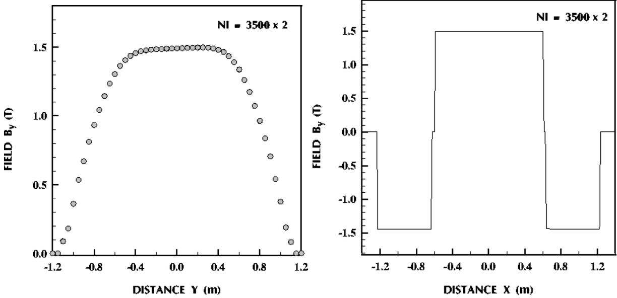
Figure 5.30: Left: Field in the prototype magnet in a direction parallel to the coil slots. Right: Field in the  $x$ -direction; the direction is reversed only outside the coils.
