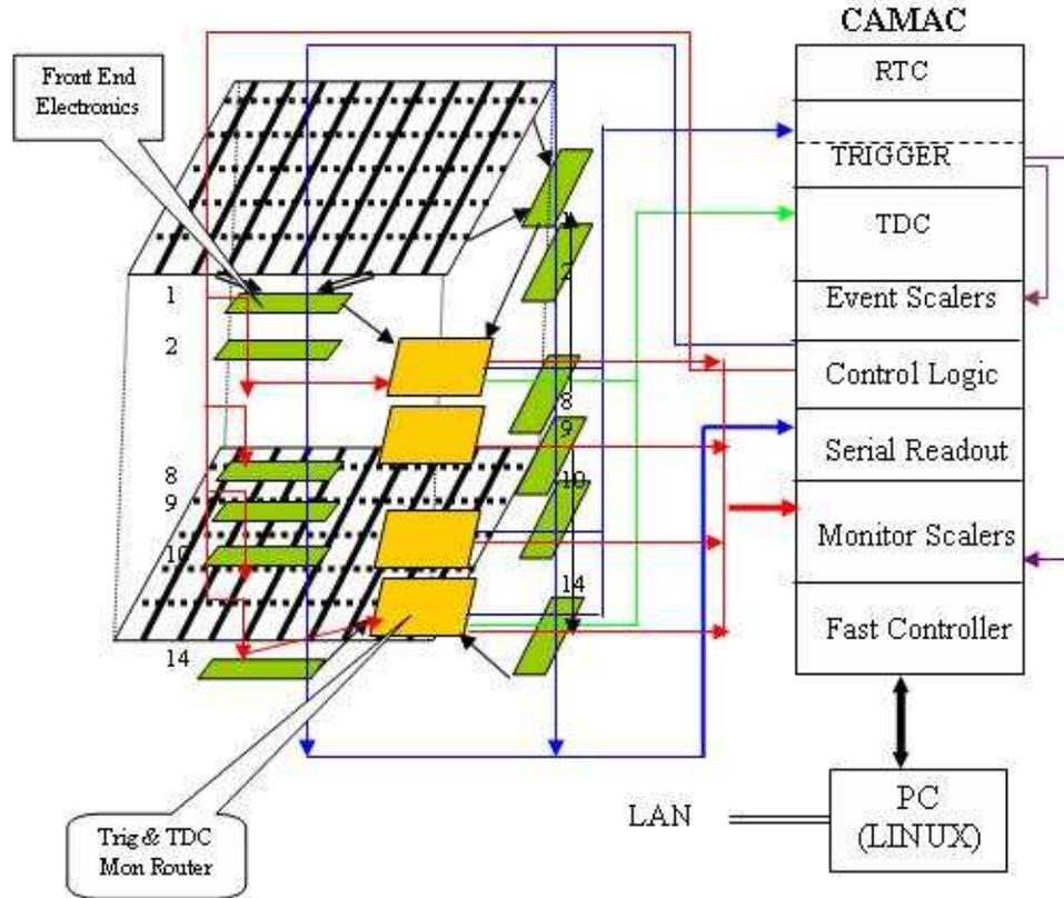
Figure 5.20: Schematic of the read-out electronics for the 1 m<sup>3</sup> prototype detector.
