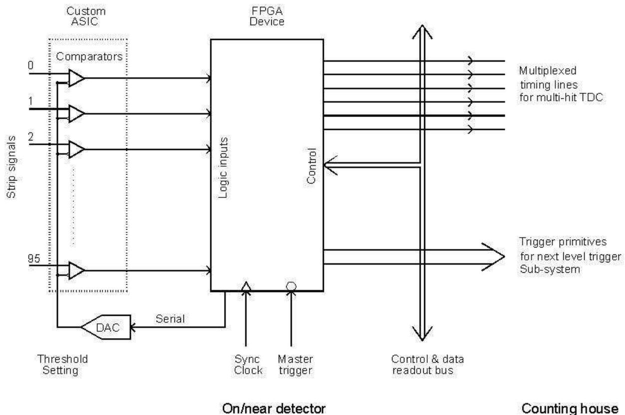
Figure 5.4: Proposed readout scheme for the ICAL detector.
