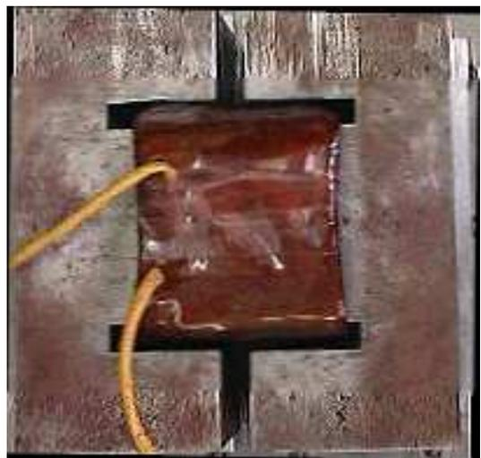
Figure 5.25: Left: Schematic drawing of the 1:100 scale model, Right: Photograph of the 1:100 model magnet with split iron pieces.
