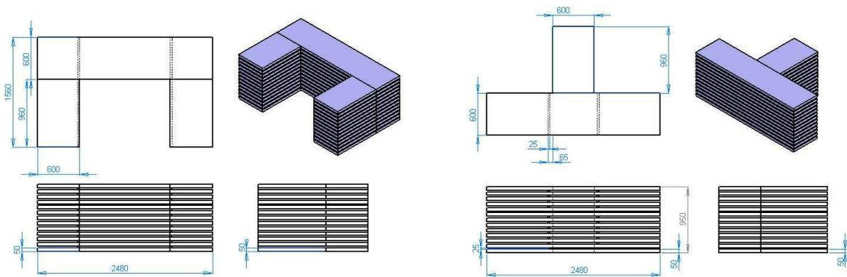
Figure 5.31: Arrangement of C-section (left) and T-section (right) of the prototype magnet.
