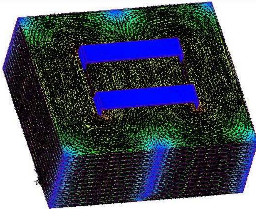
Figure 5.29: Field lines in the prototype magnet.
