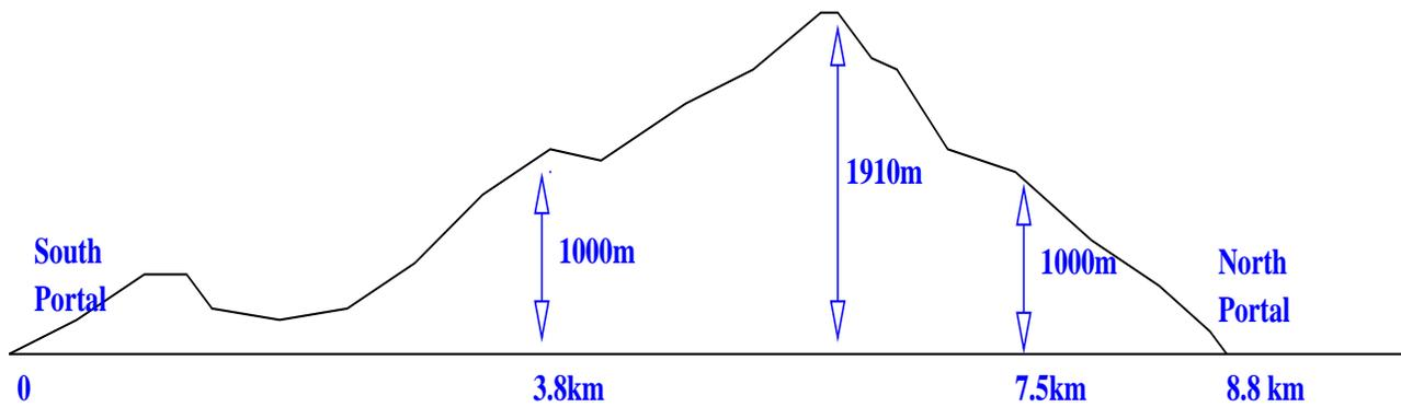
**Longitudinal Section above Rohtang Tunnel**
