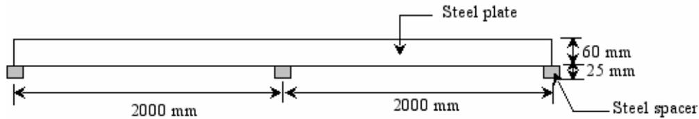
Figure 5.5: Schematic of steel structural supports for ICAL.
