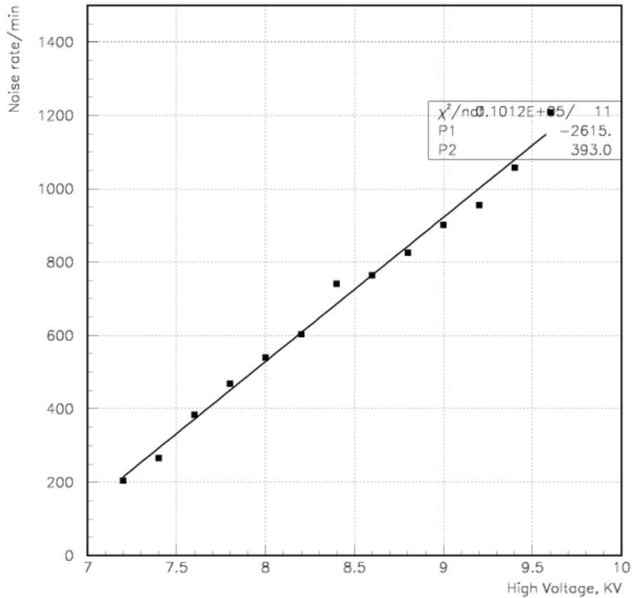
Figure 5.14: Typical noise rate plot of the RPC.
