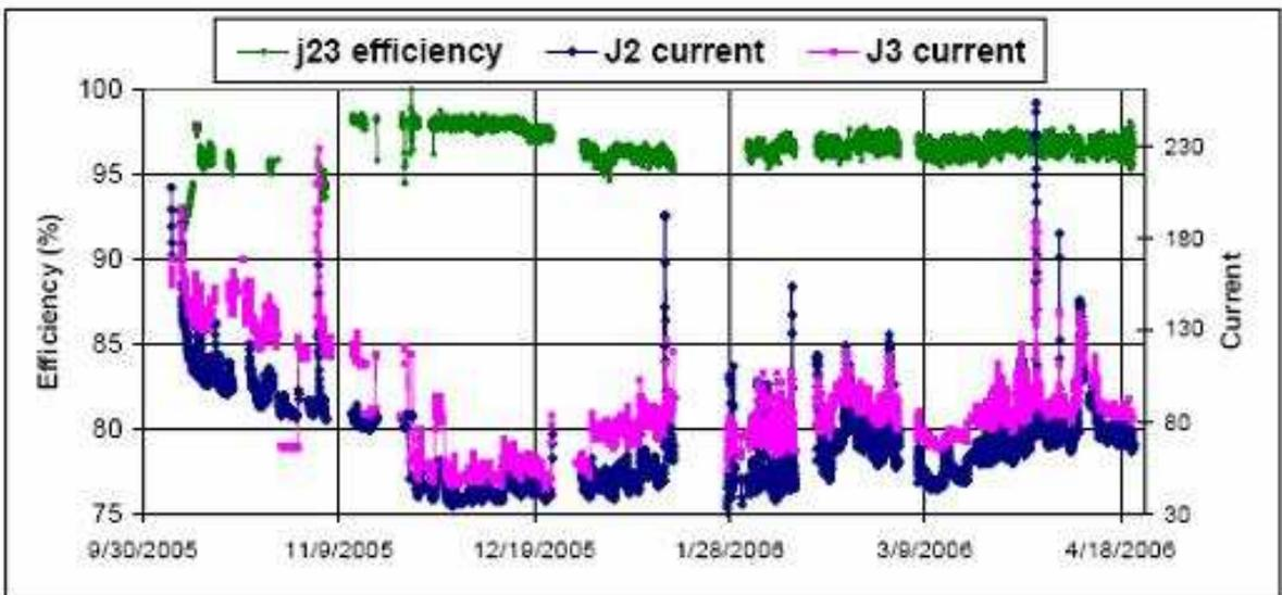
Figure 5.15: Long term stability monitoring plots of J2 and J3 RPCs.
