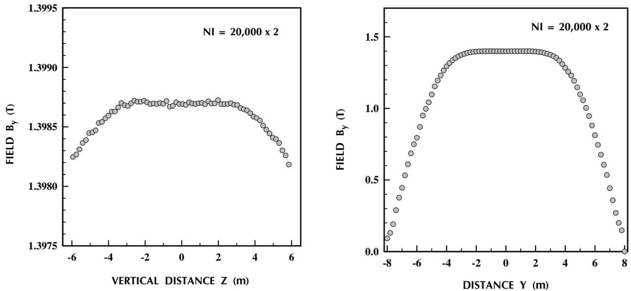
Figure 5.23: Left: Variation of field strength in z-direction, between horizontal plates. The value of NI is given in Amp.turn. Note the expanded scale. Right: Variation of field in a direction parallel to the coil slots.
