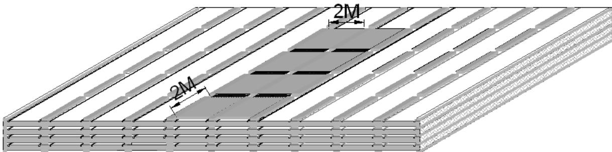
Figure 5.2: Structural detail of mounting active detector elements.
