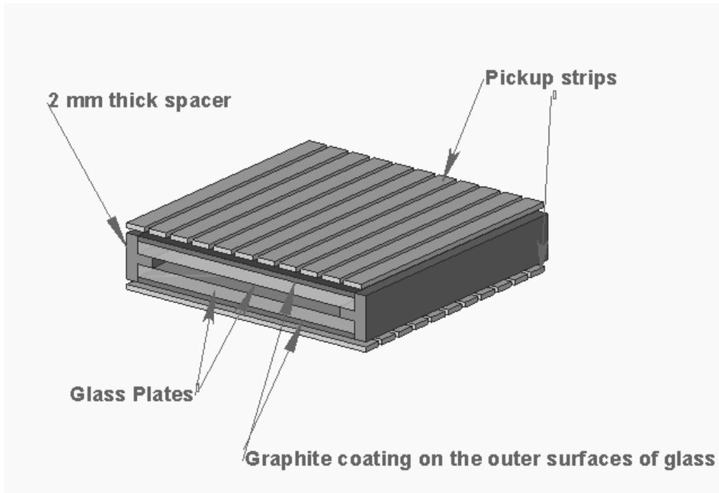
Figure 5.3: Sketch of a typical glass RPC unit.
