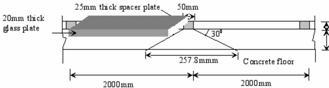
Figure C-3: Bearing width of the concrete floor.
