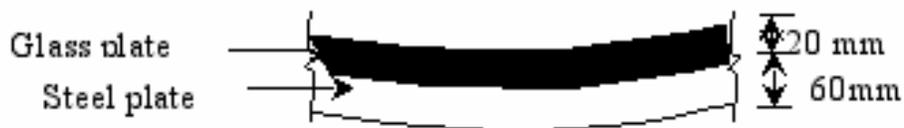
Figure C-2: Bending deformation of glass and steel.
