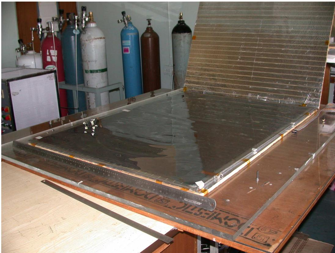
Figure 5.19: Photograph of 1 m<sup>2</sup> RPC module with its pickup strips to be used for the ICAL prototype.
