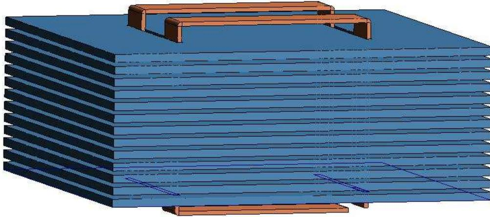
Figure 5.28: Overall view of the prototype magnet with the magnetised plates and the coil inserted. The z-axis is in the vertical direction.
