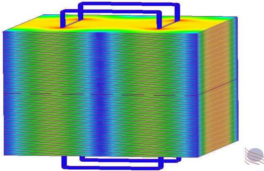
Figure 5.21: Top: ICAL magnet (three modules) showing the coil slots and the iron plate arrangement. Bottom: one module of the magnet with the coil inserted. Field uniformity can be judged by the colour pattern.
