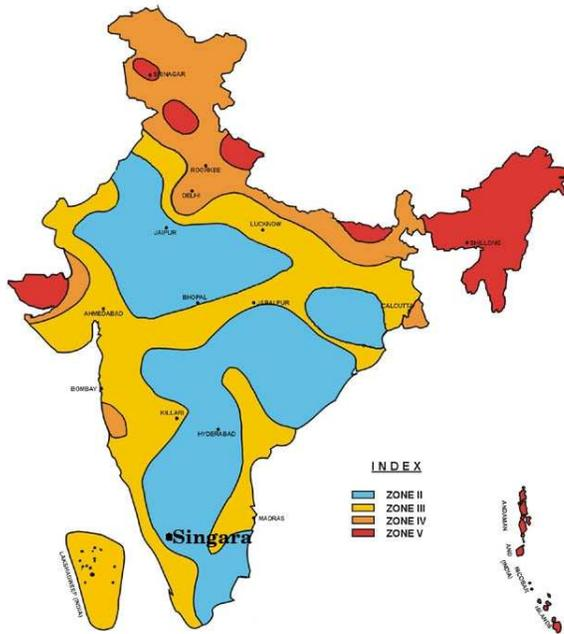
The proposed project location is in seismic zone 2 (unlike the Himalayan sites which are in either zone 4 or zone 5) which is the minimum risk zone in the country according to the zoning map (revised in 2002). Furthermore the deep underground places are often one of the safest locations when an earthquake happens. The occupied areas underground will have a refuge area in the unlikely scenario of an earthquake.
