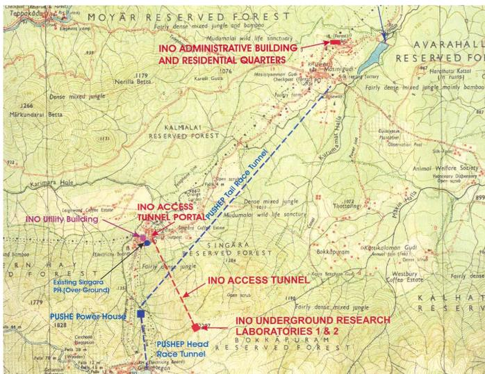
The surface facilities at the portal are minimal and include bare necessities like ventilation, cooling and power systems. The laboratory will be serviced along the single access tunnel for all its requirements. The air-blowers situated at the entrance provide fresh air through the tunnel with its outflow being at the portal itself. The present design does not include shafts or vents at any point along the tunnel.
