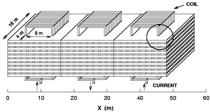
Neutrinos will interact with the iron material of the detector to produce charged particles. The iron layers will be sandwiched with the active detector material that will detect whenever a charged particle passes through it. The ICAL detector will consist of three modules of 16 kton each.
