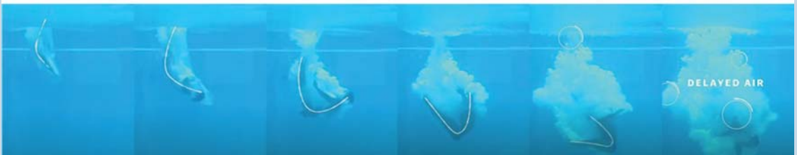
Delayed breaking of entrapped bubbles into smaller bubbles by turning
