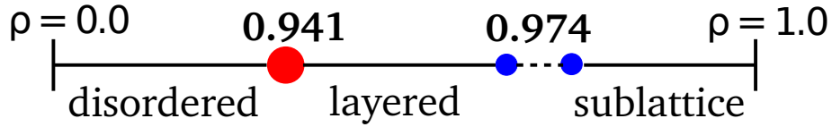
Figure 4.12: Schematic phase diagram of 2 \times 2 \times 1 hard plate model. Red dot represent second order transition and dotted line represent first order transition.
