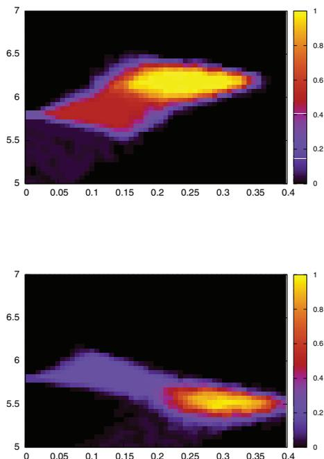
Fig. 2: (Colour on-line) Probability of obtaining logic operations (see text): (top)  $P(\text{NAND})/P(\text{AND})$ ; (bottom)  $P(\text{NOR})/P(\text{OR})$ . The  $x$ -axis displays noise intensity  $D$  and the  $y$ -axis displays  $\gamma$ .
