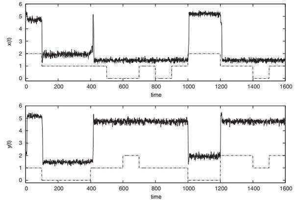
Fig. 9: Time series of  $x(t)$  (upper panel) for AND gate and  $y(t)$  (lower panel) for OR gate, with  $D = 0.3$  in the case of independent input sets. The dash-dotted lines show the inputs  $I = I_1 + I_2$  (upper panel)  $I' = I'_1 + I'_2$  (lower panel). The upper panel shows consistent AND (taking  $x > 3$  as output 1;  $x < 3$  as output 0) response most likely, and the lower panel shows OR response in the same threshold.
