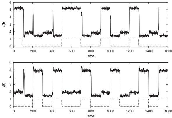
Fig. 8: Time series of  $x(t)$  (upper panel) and  $y(t)$  (lower panel), with noise intensity  $D$  equal to 0.3. The dashed line shows the desired logical outputs (AND for the upper panel and XOR for the lower panel). Almost certainly, the upper panel shows consistent AND (taking  $x > 3$  as output 1;  $x < 3$  as output 0) response, and the lower shows XOR response in the same threshold.
