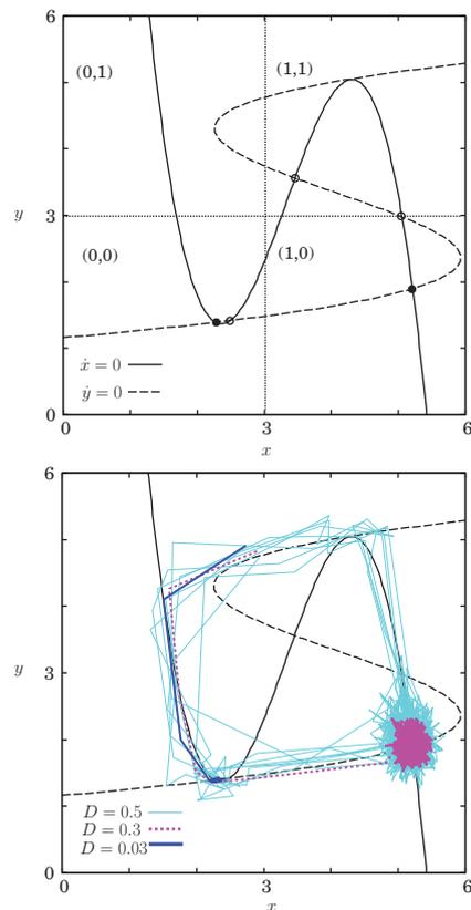
Fig. 7: (Colour on-line) Top: null-clines for the system (5) and (6) in the phase space, for  $(I_1, I_2)$  equal to (1, 1). Corresponding pairs of logical outputs are indicated in the region segmented by the dotted lines. The open circles are the unstable fixed point and the filled circles are stable ones. Bottom: three trajectories for  $D = 0.03$ ,  $D = 0.3$  and  $D = 0.5$  are shown.
