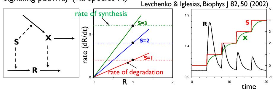
Perfect adaptation: Although the signaling pathway exhibits a transient response to changes in signal strength, its steady-state response
