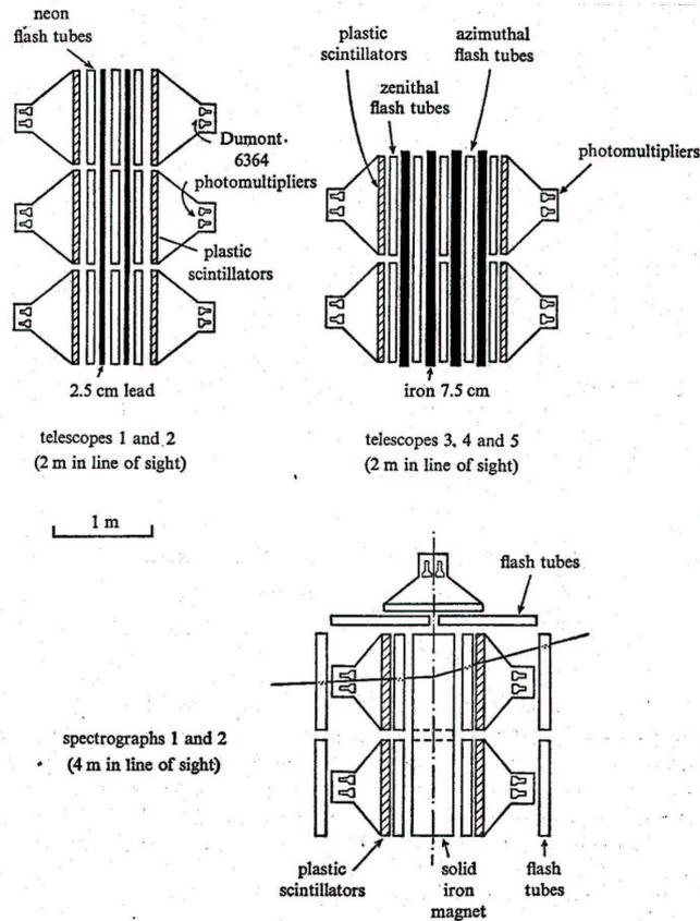
Fig. 4 Neutrino detectors at the depth of 2.3 km at KGF
