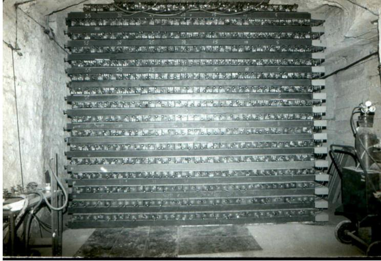
Fig. 12 Front view of Phase 1 Nucleon decay detector at 2.3 km depth in KGF. Each square section seen here is of a proportional counter giving a grid size of 10 cm × 10 cm.
