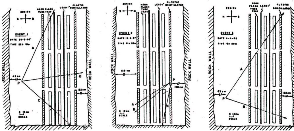
Fig. 7 Multi-track (Kolar) events recorded in KGF neutrino-detectors.
