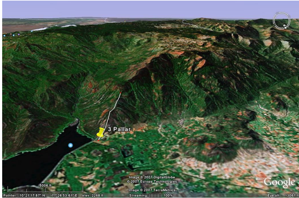
The Google Earth image shows the site Palar 3 with projection on the terrain of a tunnel 2500m long and overburden of 628m.
