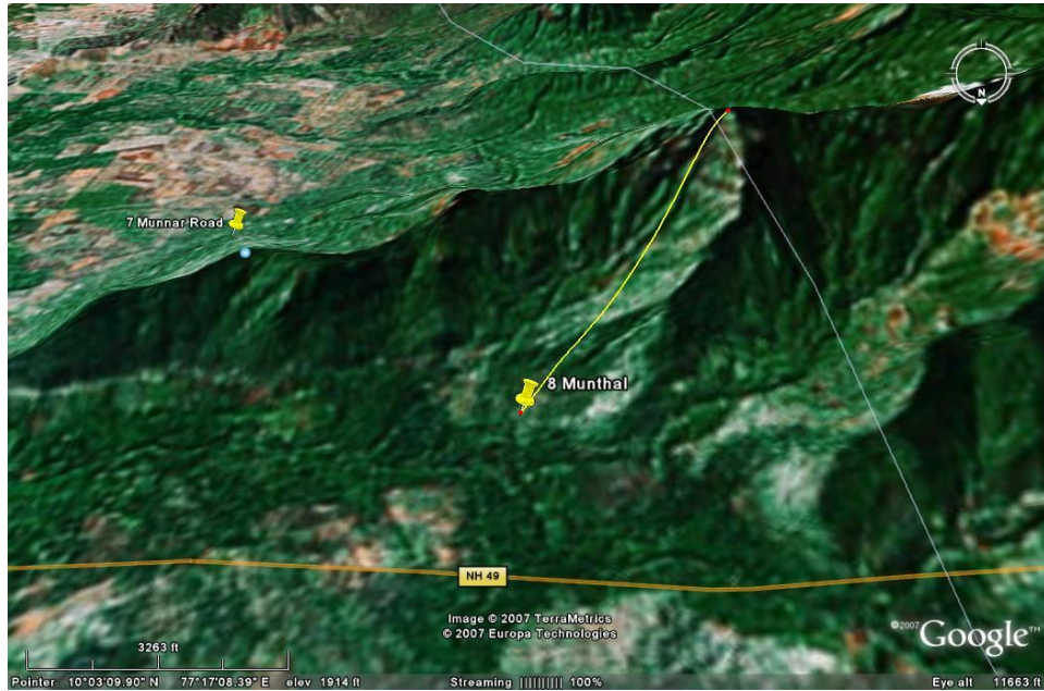
The Google Earth image shows the site Munthal 8 with projection on the terrain of a tunnel 1870m long and overburden of 846m.
