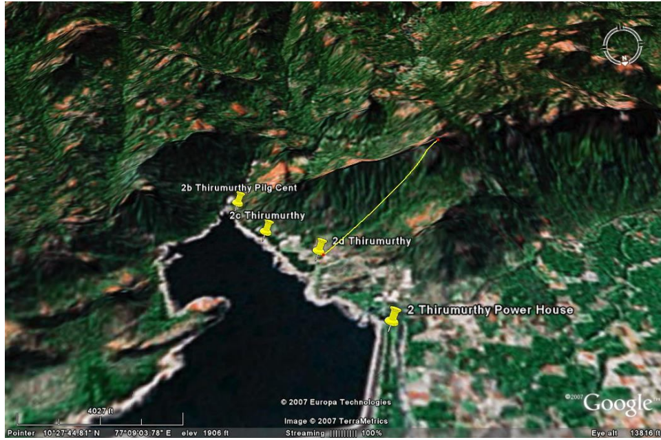
The Google Earth image shows the site Thirumurthy 2d with projection on the terrain of a tunnel 1720m long and overburden of 664m.
