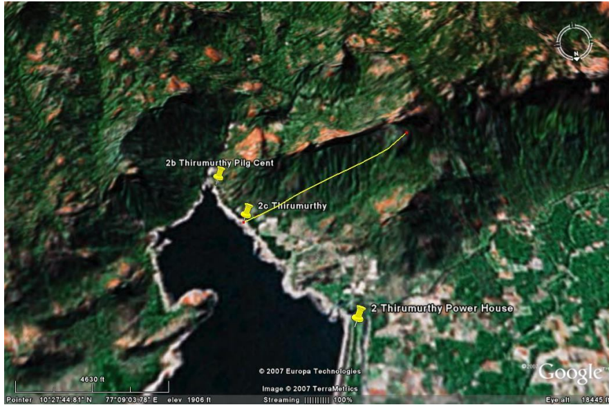
The Google Earth image shows the site Thirumurthi 2c with projection on the terrain of a tunnel 2000m long and overburden of 630m.
