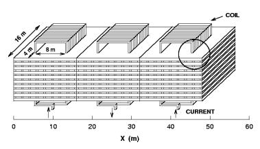
Neutrinos will interact with the iron material of the detector to produce charged particles. The iron layers will be sandwiched with the active detector material that will detect whenever a charged particle passes through it. The ICAL detector will consist of three modules of 16 kton each.
