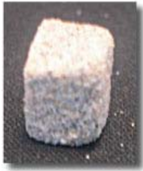
Sandstone specimen (may be from disintegrated core material or drill cuttings)
